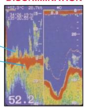
The bottom is displayed as a straight line. Echoes immediately below this line will have enhanced bottom tails. Harder bottom creates darker and longer tails. The nature and any changes in bottom density can be easily determined by any changes in color or tail lengths.
